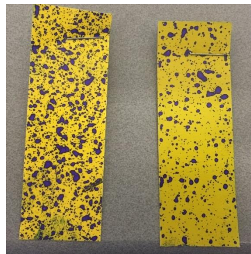
Figure 8. 100L/ha of water on the left vs 50L/ha of water on the right. Both very coarse droplets.
