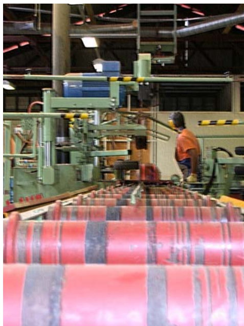
Plate 1: DPI&F's Kara saw processing a K. senegalensis log. Milling room.
