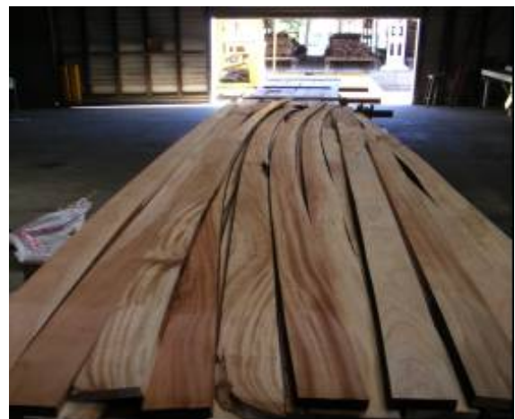
Boards with excessive spring
