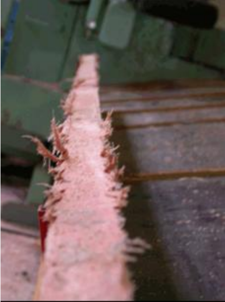
Plate 12: 'Woolly edge' to a GOS board, indicating interlocked grain
