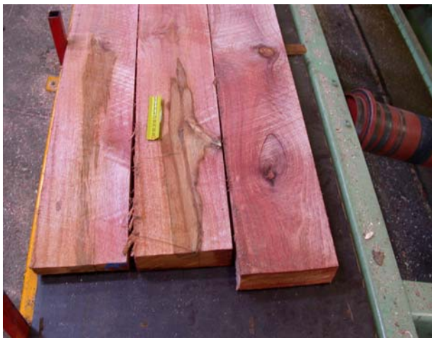
Plate 15: Decay in the inner heart, which has entered via a rotten branch stub, across three boards cut consecutively from a cant.
