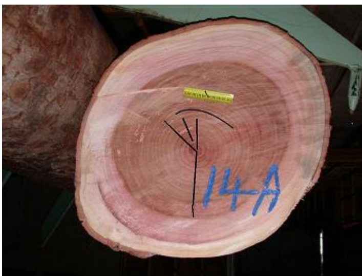
Plate 7: Log end-splits (splits highlighted)
