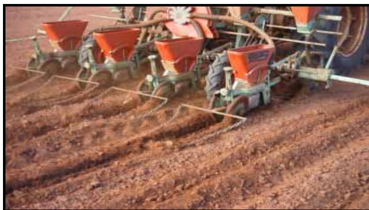
Figure 10. A Nodet Gougis vacuum planter, capable of banding fertiliser below and beside seed
