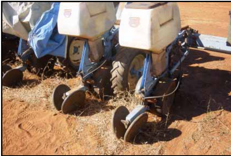
Figure 1. Press-wheels such as “twin inclined” will assist germination on red soils provided the surface remains moist until emergence
