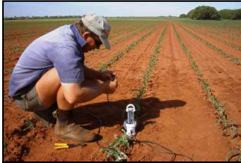
Figure 30. Installing an Enviroscan® in a maize crop
