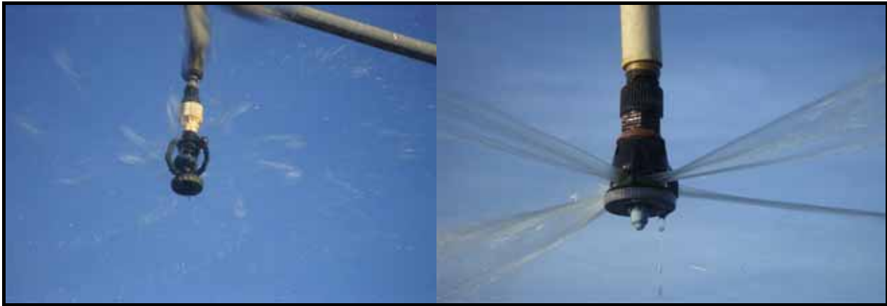
Figures 32a and b. Different sprinkler heads will give different efficiencies. Wobbler type sprinklers (left) reduce drift and evaporative losses in high winds and hot conditions.
