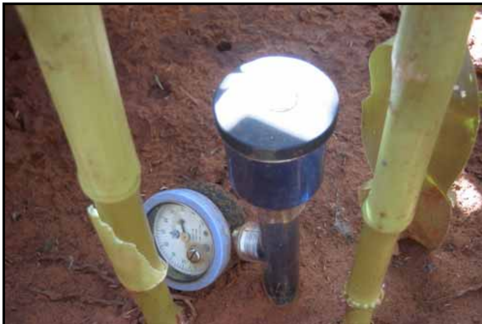
Figure 9. Jetfill® tensiometer used to assist in scheduling irrigation for maize
