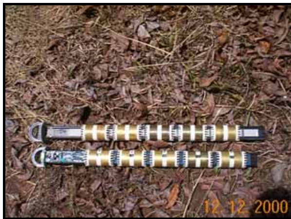
Figure 29a and b. Enviroscan® capacitance sensors and data logger
