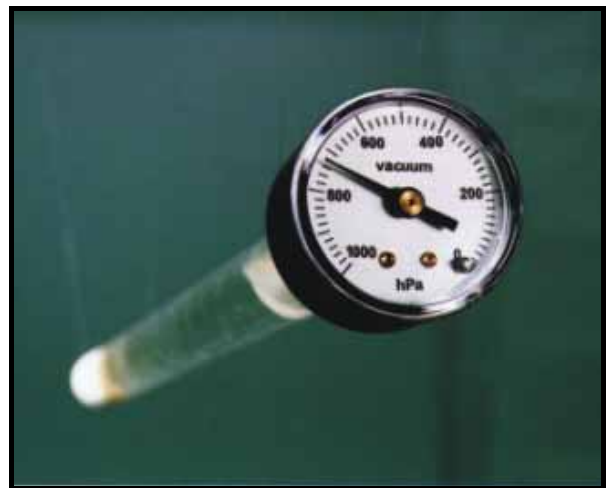
Figure 31a. Tensiometers at different depths in a peanut crop and b. Tensiometer with gauge
