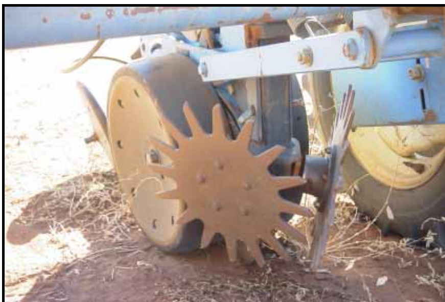
Figure 26. Row sweepers on a conservation tillage planter, which “sweep” the row clean of mulch to allow the seed to be planted without obstruction
