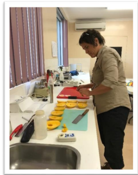
Figure 7. Dallas Anson cuts a careful section of flesh to place under the probe of a texture analyser, then extract juice from the remaining flesh to measure sugar content.
