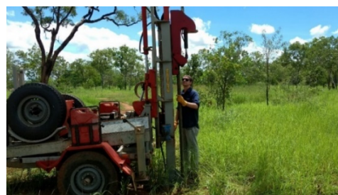
Image: Patrick Burly demonstrating DENR's hydraulic soil sampling drill
