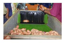
multiple high pressure spray jets. Harvested roots are immersed in the water hopper which lessens skin rubbing damage and loosens soil adhering to the roots before entering the washing brushes. Avoid hard brushes which can damage the skin and clean brushes and conveyors regularly to avoid latex build-up.
