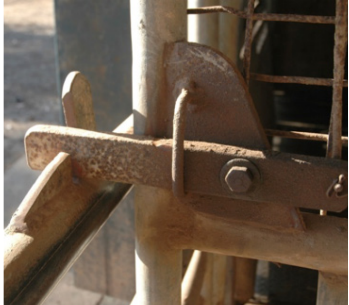
Figure 11.9 Close-up of locking latch which engages automatically when the gate is swung closed.
