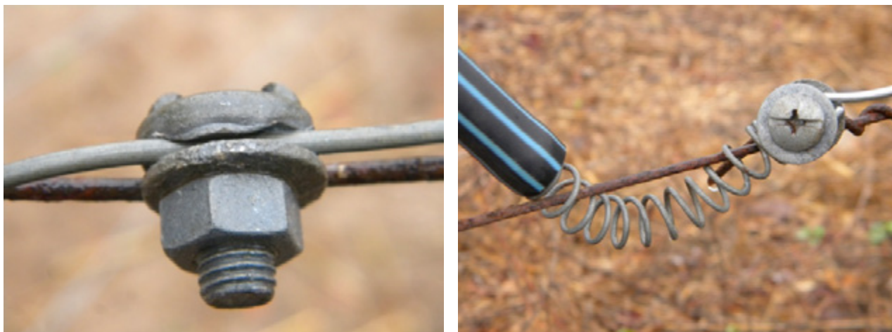
Figure 11.3 Permanent connector (left) and curl-on or (pig tail) connector (right). The alternative to the curl-on is a more expensive on-off switch. The high tensile spring gives a good connection for current, particularly when the fence wire is not rusty!
