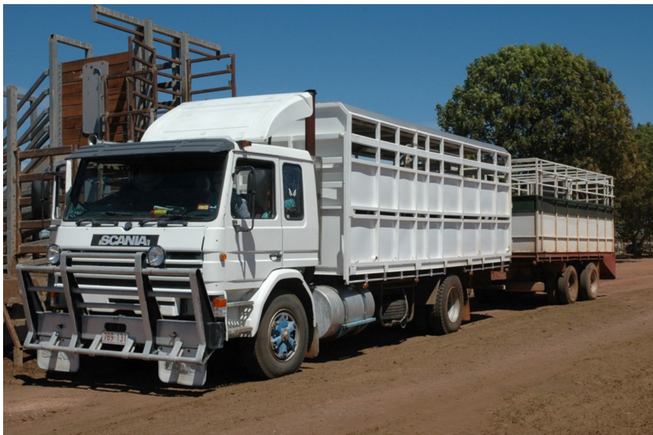
Figure 6.1 Trucks need to be equipped with sturdy crates for protection of transported stock.
