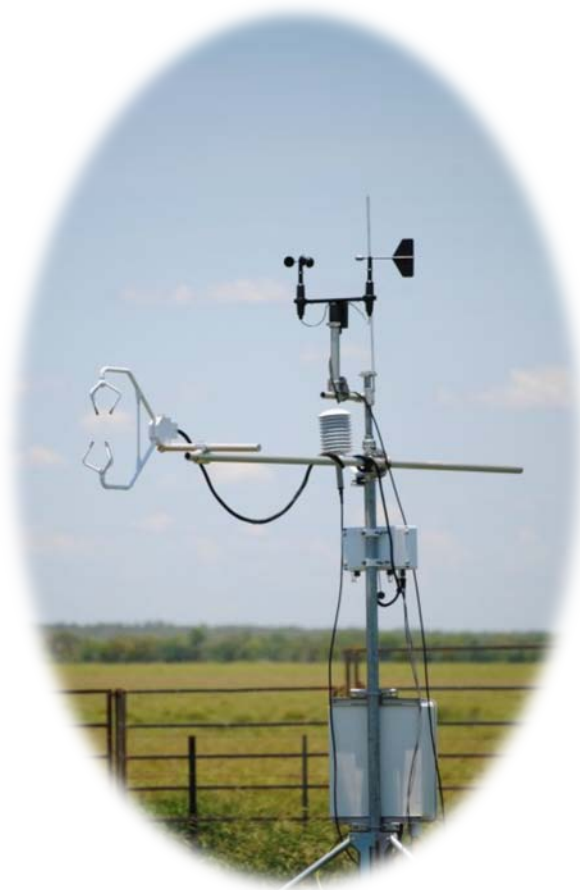
Figure 16. Mobile weather station used during a study of methane production from grazing cattle
