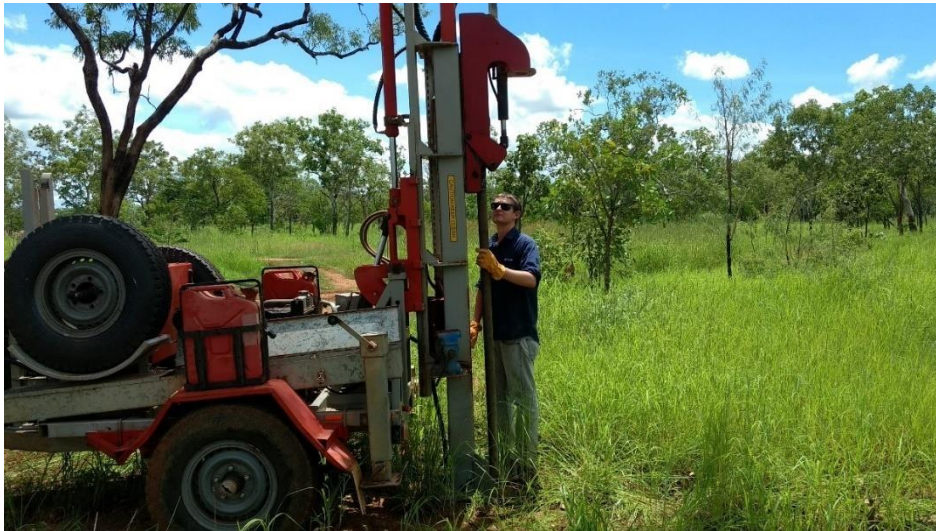
Above: Patrick Burly of DENR demonstrating the use of their hydraulic soil sampling drill
