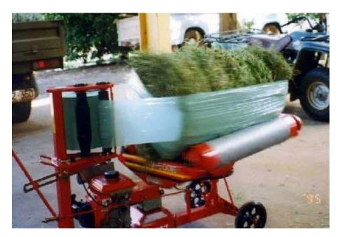
Figure 3. A small bale wrapper in operation
