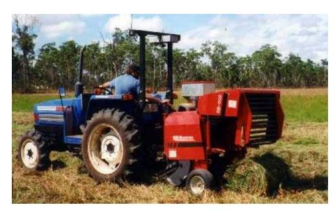
Figure 1(b). A variable chamber baler forming small round bales
