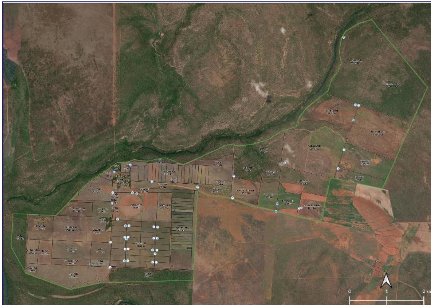
Map 2. Douglas Daly Research Farm (August 2024), including troughs (T), bores (B), dams (D), water tanks (W) and paddock layout and names.
