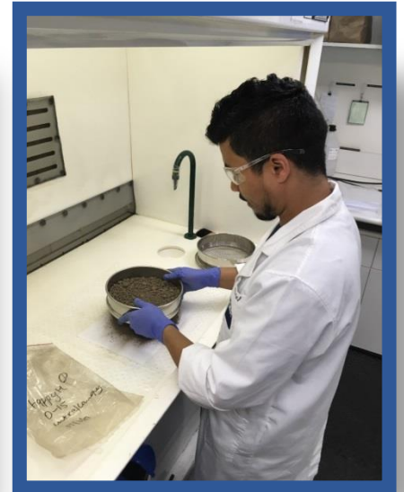
Figure 7 QUT PhD student Raj Pandeya sieves a 'mango' soil from the Darwin Region
